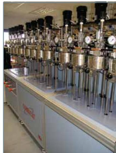
12 x High Pressure Glass Reactors, C276, Hydrogenation and with hydrogen dosing, 200 bar, 250 C.
