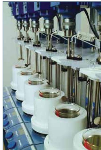
6 x Low Pressure Glass Reactors. For Testing Lubricants, 250 C.
